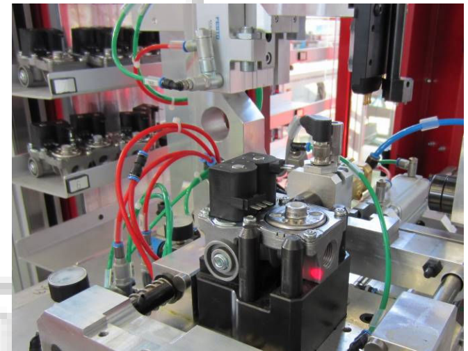
Automatic testing station, automatic loading unloading, repairing rack for defective valves.
