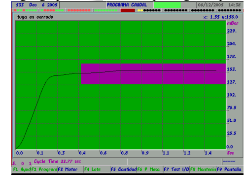
Leak test real time graphics.
